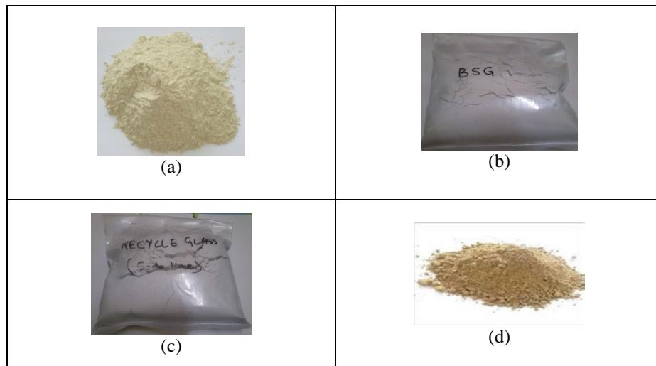
Figure 1.1: Type of materials used in this project a) Bentonite powder, b) Borosilicate glass (BSG), c) Soda-lime glass (SLG) and d) Spent Bleaching Earth (SBE) (Vasundhara Industries, 2011; Cargo Handbook.Com, 2013).
