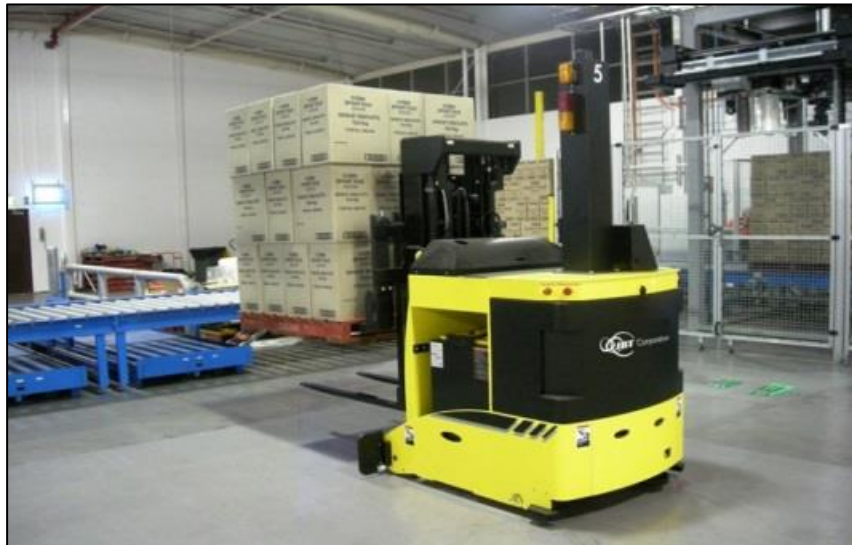
Figure 1.2 : Example of Automated Guided Vehicle.
