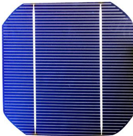
Figure 2.2: Monocrystalline solar panels
