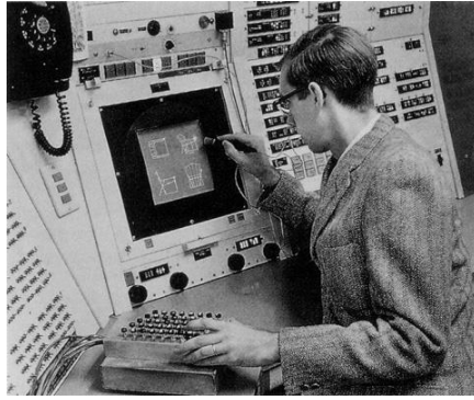
Figure 1.1: Sketchpad software console developed by Ivan Sutherland (1963)
