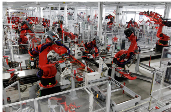
Figure 2.5 : Fixed or hard automation assembly method
