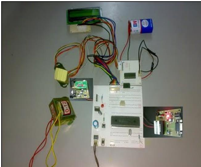
Figure 2.1: RFID and GSM Mail Box
