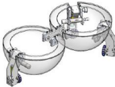
Figure 2.4: Reconfigurable robot after transformation
