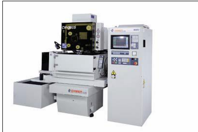
Figure 2.3: Example of EDM Wire Cut (Moulton et al. 2013)
