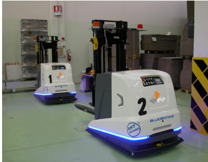
Figure 2.1: Autonomous guided vehicle system in a factory ( www.bluebotics.com )
