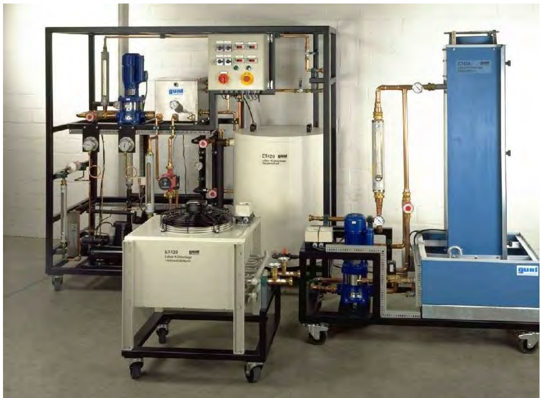
Figure 1.1: Ice store in refrigeration system
