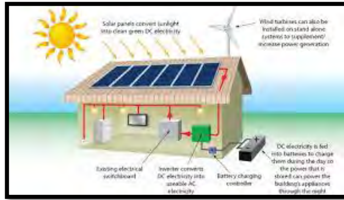
Figure 2.2: Stand-alone PV system working principle
