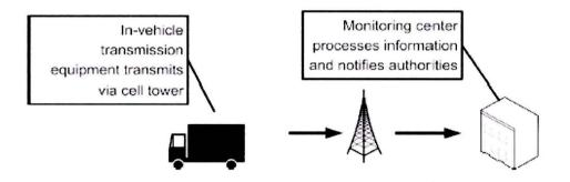
**Figure 2.1 Traditional Accident Detection System**
