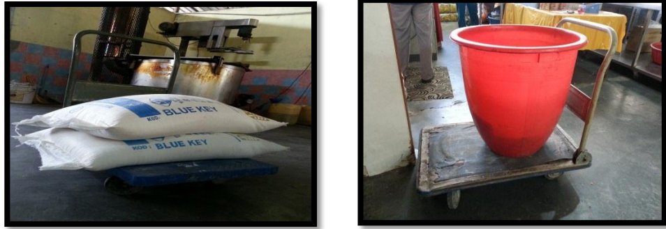
Figure 1.1: The overloaded materials and inappropriate usage of material handling
