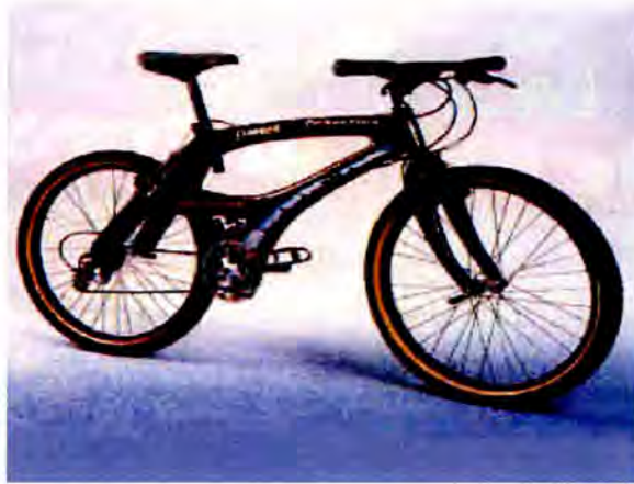
Figure 1.4 The bicycle frame is made of glass-carbon reinforced epoxy (Copyright © 1996-98 Torben Lenau).
