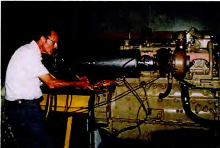
Figure 2.5: 1 kW generator mounted on Cummins NTC 350 engine [2]
