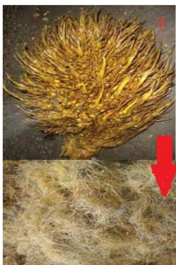
Figure 1.1: Empty fruit bunch and the processed fibre (Rozman et al.2003)
