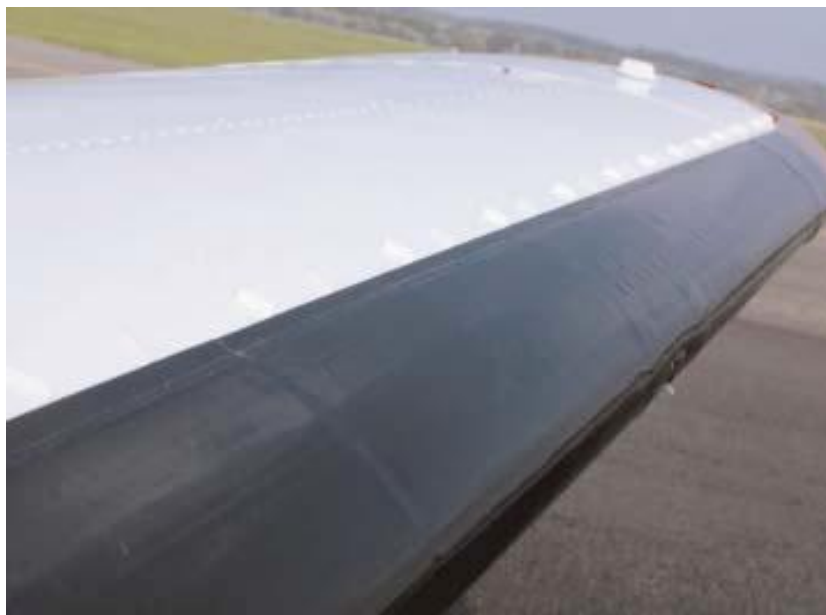
Figure 2.3: Pneumatic De-icing Boot (Source: Murphy and Bell (2004))
