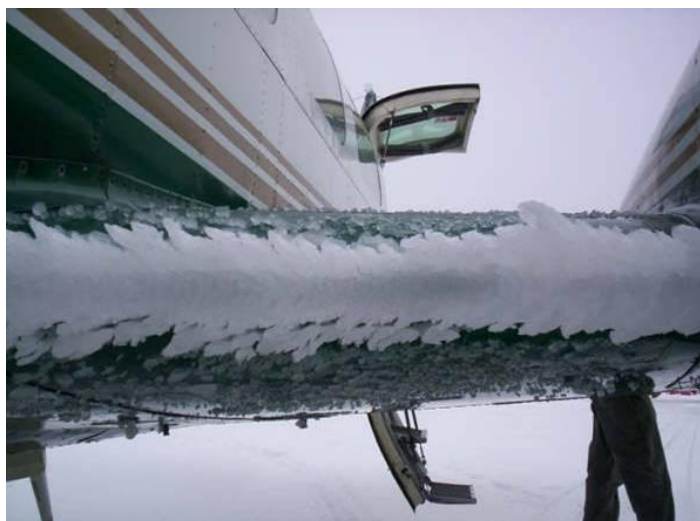
Figure 2.2: Aircraft with ice formation on land (Source: Meteorology-Part II [Active Weather] Website, Retrieved on 30th November 2012)
