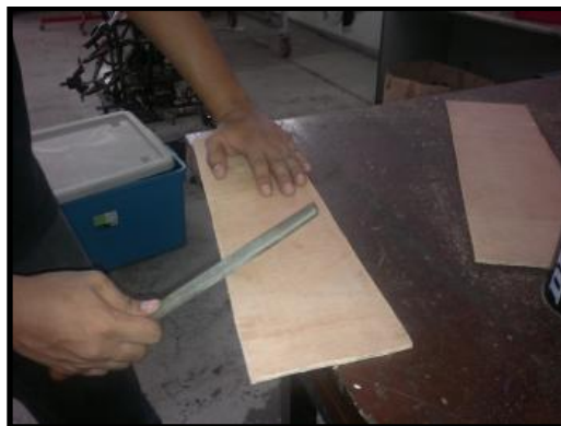
Figure 3.9: Finishing the plywood
