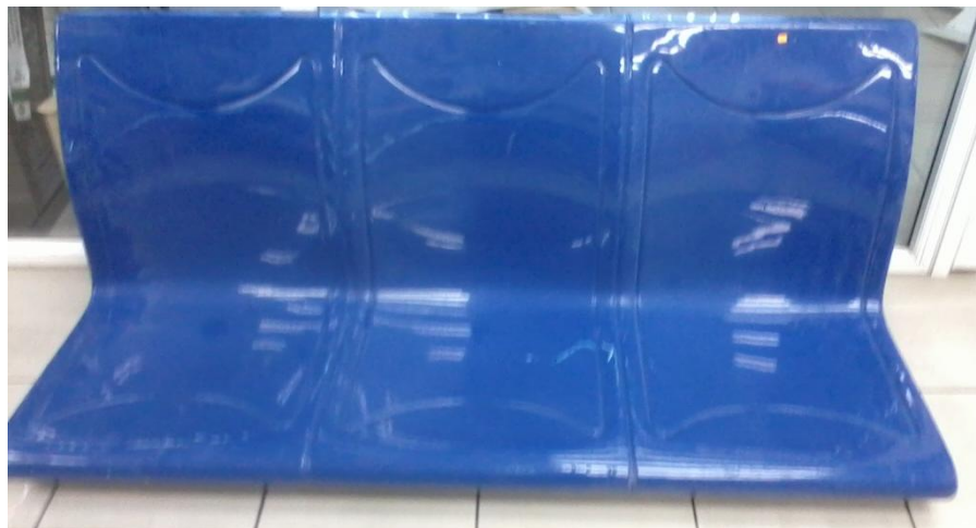
Figure 2.3: Application of FRP on rail seat
