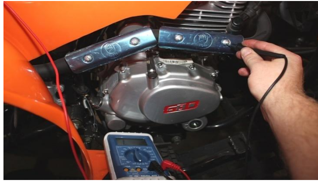
Figure 2: Check the connectivity of ignition circuit by using multimeter (Geobikes.com)
