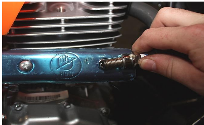
Figure 1: The typical way of a motorcycle user to check the spark of spark plug (Geobikes.com)
