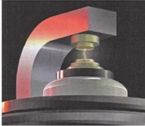
Figure 5: A spark on the spark plug (Abdo, 2012)
