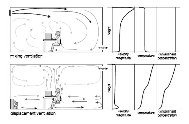
Figure 2.1: Schematized Representation of Mixing and Displacement Ventilation Principle; Flow Pattern (left) and Variable Gradient of the Height (right). At a given Height the Variable has been Averaged over the Total Horizontal Plane in the Room (Loomans, 1998).
