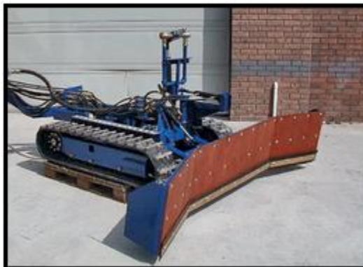
Figure 2.2 : Oil Tank Sludge Cleaning Robot
