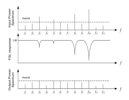
Figure 2.1: Performance of a frequency selective limiter [1-4]
