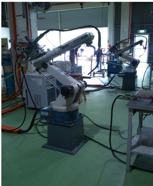
Figure 2.1: Arc welding robot (GMAW),(UTeM,FKP Laboratory)
