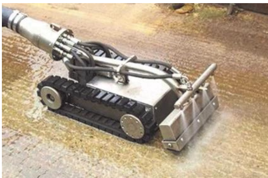
Figure 2.3: Remote Tank Cleaning, RTC. (Photograph reprinted from Tank & Pipework Ltd. 2011)
