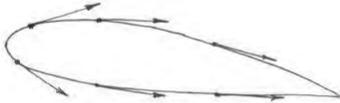
Figure 2.3: Shear Stress Distribution (Source: Bray, 2003)
