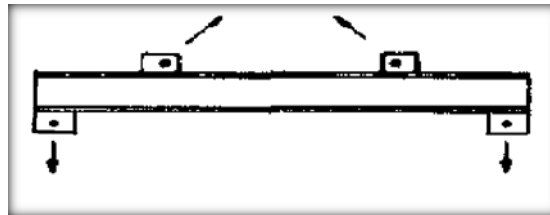
Figure 2.2: Spreader beam with two upper lifting lugs (David, 2003)
