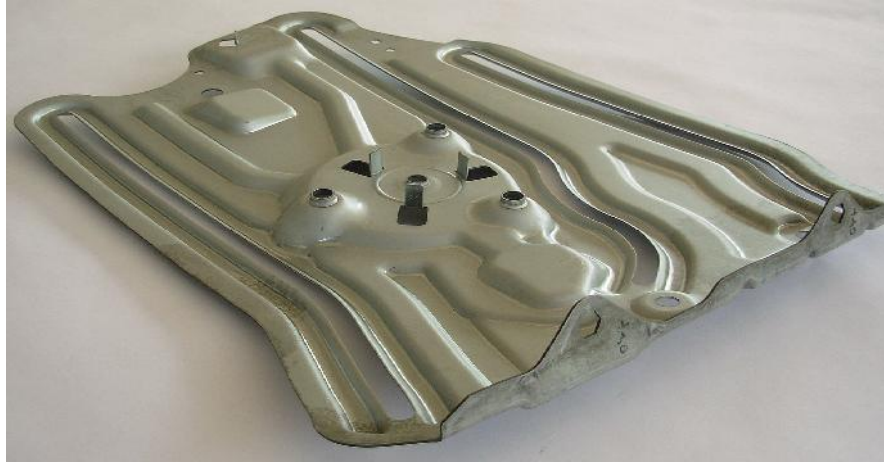
Figure 1.1: Complex part of drawing process – Automotive plate
