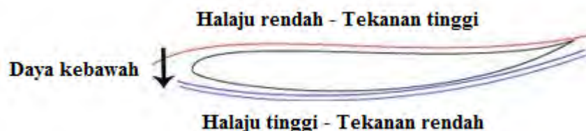
Rajah 1.4 : Daya kebawah, prinsip Bernoulli (Sumber: www. racecarengineering.com )
