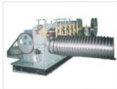
Figure 1.2: Rolling machine in fabricating screw.
