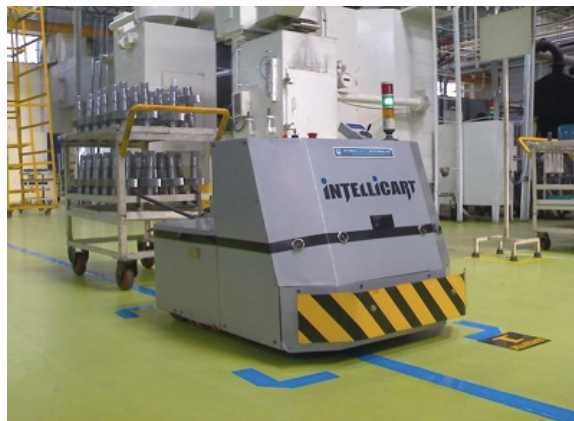
Figure 1.0: Automated Guide Vehicle (AGV) towing trolley. (Designed by: Hi-Tech Robotic Systemz Ltd, India).
