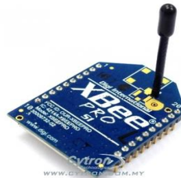
Figure 1.6: XBee Pro 60mW Wire Antenna (Source: < http://www.cytron.com.my >)
