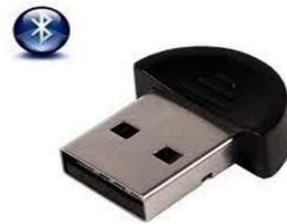
Figure 1.5: Mini USB 2.0 Bluetooth Dongle (Source: < http://www.basco.com >)
