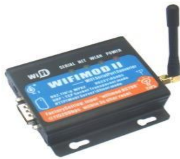
Figure 1.4: WIFI moduleSerial (RS232) (Source: < http://www.toboc.com >)
