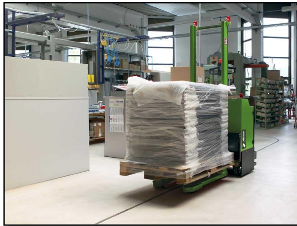
(c) AGV forklift trucks.
