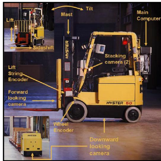
Figure 2.5: Structure in AGV system (Arkin, 1989).
