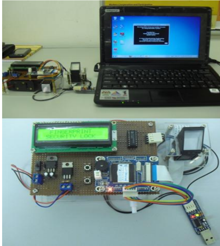
Figure 1: Hardware setup consists of an off-shelf-product (below) that was used to register a user, whose fingerprint data was saved in a PC system
