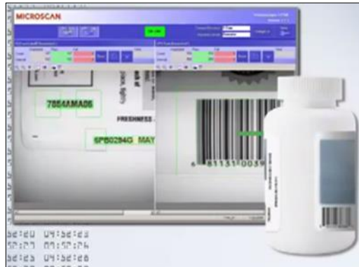
Figure 1.7: Decoding application by using vision system (Microscan System Inc, 2012).
