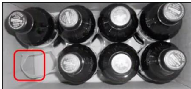
Figure 1.3: Counting application of vision system, (Microscan System Inc., 2012).
