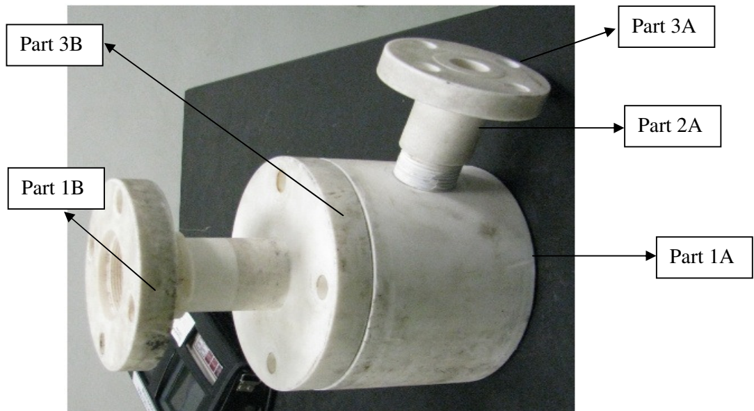
Figure 1.3: Existing Part of Ejector [Petronas (2012)].
