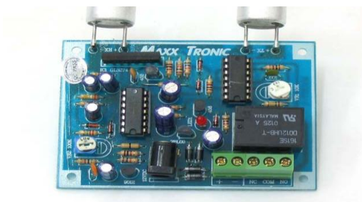
Figure 2.3: Ultrasonic Sensor Module Components
