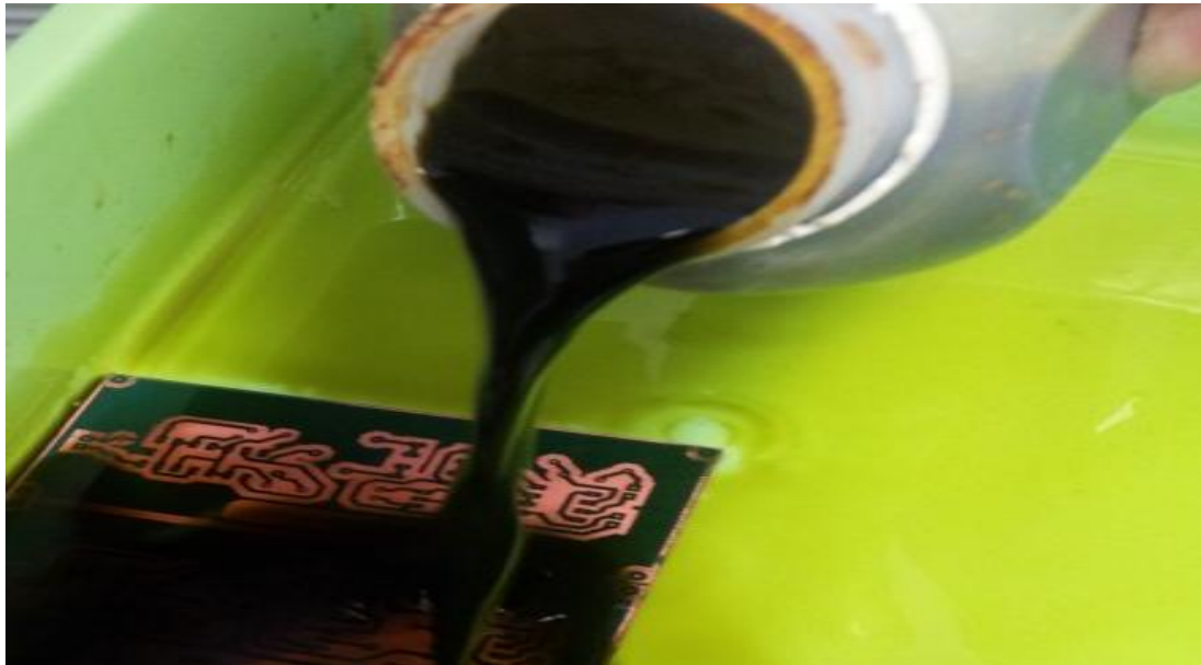
Figure 3.11: Etching the PCB
