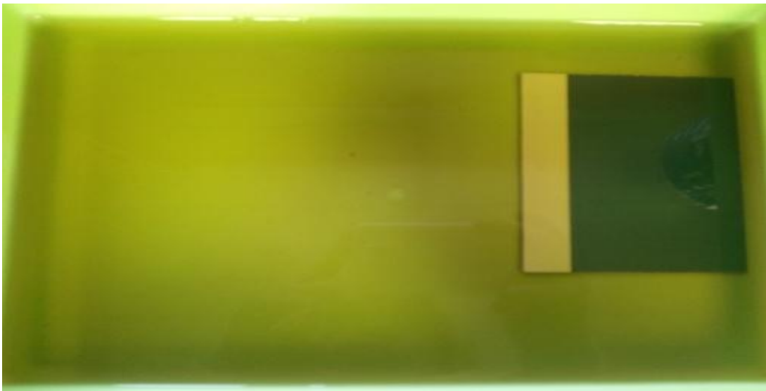
Figure 3.10: Developing the PCB
