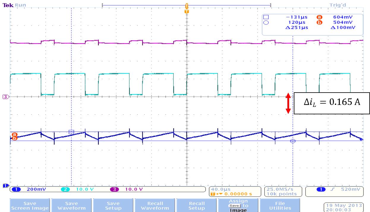
Figure 4.36: Pulse with a duty cycle, D of 70% and the current ripple, i_L at the inductor
