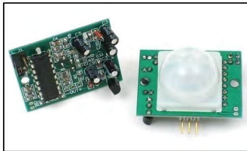
Figure 2.4: Passive Infra-Red (PIR)
